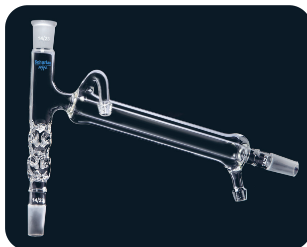
MICRODISTILLATION WITH LIEBIG CONDENSER, OUTLET WITH NS CONE, WATER CONNECTION WITH OLIVES, WITH SOCKETS NS 14/23
