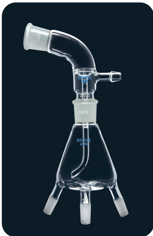
DISTILLING RECEIVERS, ACC. BREDT, BENT, FOR FOUR FLASKS NS, WITH BENT ADAPTER (105°) AND VACUUM CONNECTION
